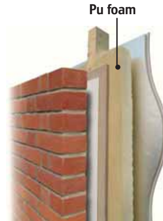
Timber frame wall
